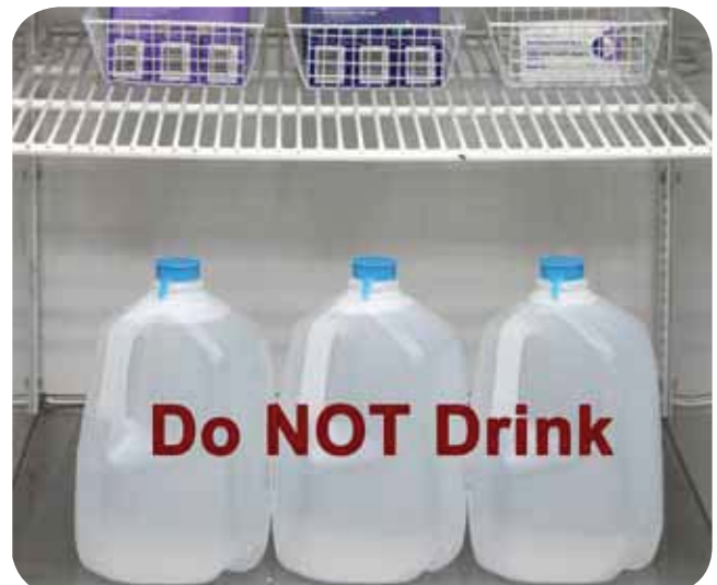
Stabilize temperature in a refrigerator with water bottles labeled “Do NOT Drink.” Stabilize temperature in a freezer with frozen coolant packs.
