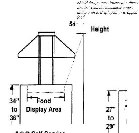
1. If a single unit **Agent Series Series**, the ends of the unit must be closed to prevent consumer access to unprotected food. Otherwise, units must be in line with other equipment to prevent access from unshielded sides.
