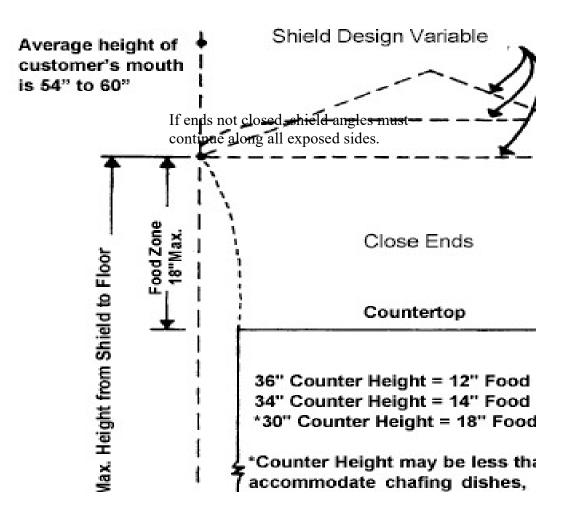
*Note: Ends must be closed. Otherwise, units must be in line with other equipment to prevent access from unshielded sides.*
