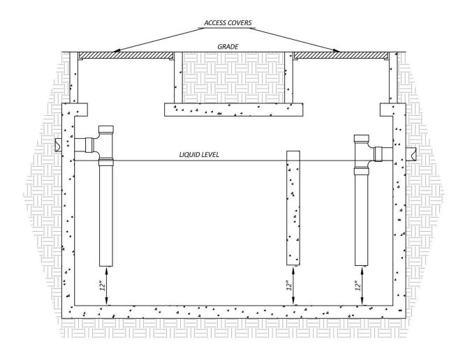
Figure 9.D Septic Tank to Grease Trap Conversion
