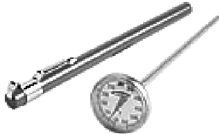
“Bimetallic Stemmed Thermometer” Not accurate to probe thin foods
