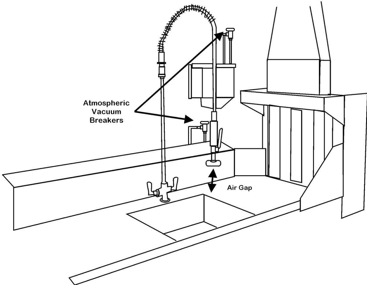
*This is a typical warewashing machine installation where atmospheric vacuum breakers can be easily seen.*
