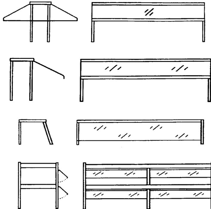
**Note:** If a single unit is being used for self-service, the ends of the unit must be closed to prevent consumer access to unprotected food. Otherwise, units must be in line with other equipment to prevent access from unshielded sides.
