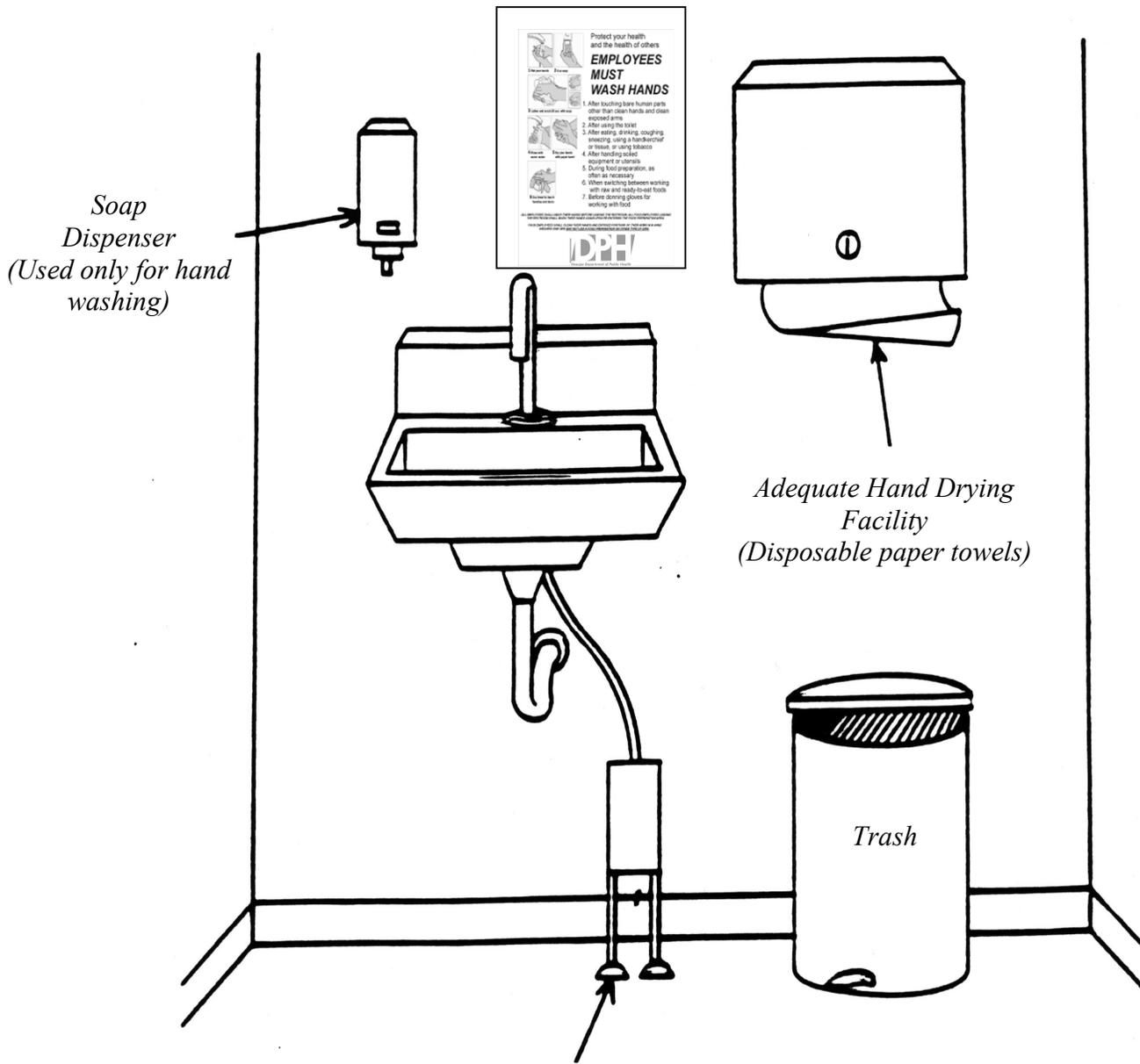
*This foot-peddle fixture can be replaced with standard mixing valve faucet.*
