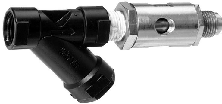
*A dual check valve with an intermediate vent preceded by a screen of not less than 100 mesh to 1 inch shall be installed upstream from a carbonating device and downstream from any copper in the water supply line. This requirement in DPH Chapter 511-5-14 is more stringent than ASSE 1022 for use on a carbonator. The 100 mesh screen is not part of the ASSE standard for carbonator protection.*
