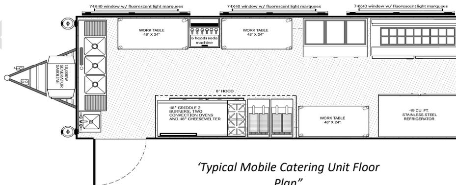
*“Typical Mobile Catering Unit Floor Plan”*
