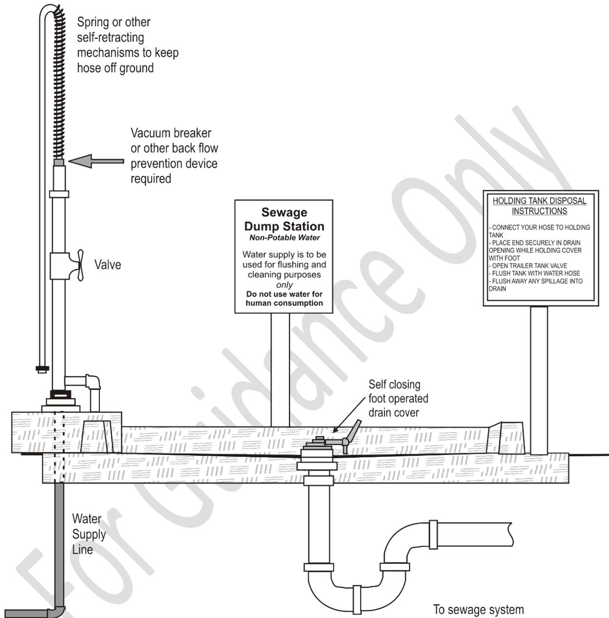
*Note: Waste piping will be not less than four inches in diameter unless specified by applicable law or local codes.*
