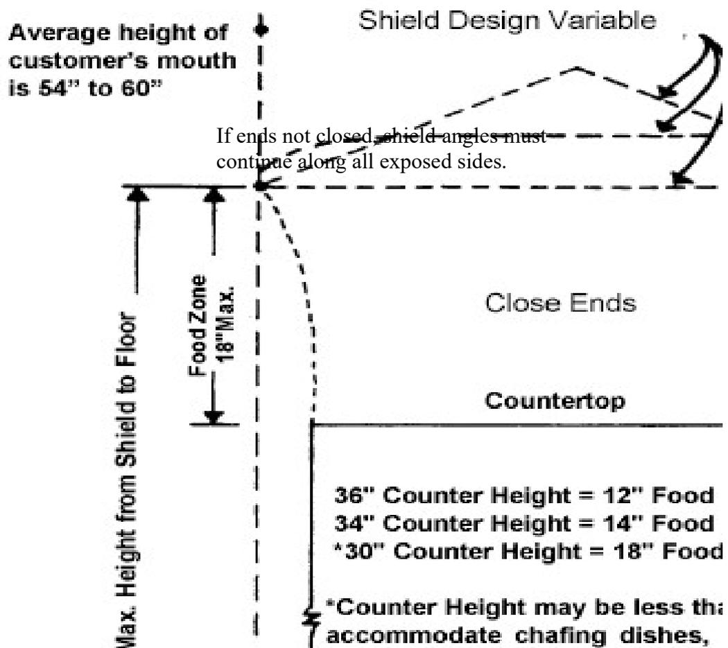
*Note: Ends must be closed. Otherwise, units must be in line with other equipment to prevent access from unshielded sides.*
