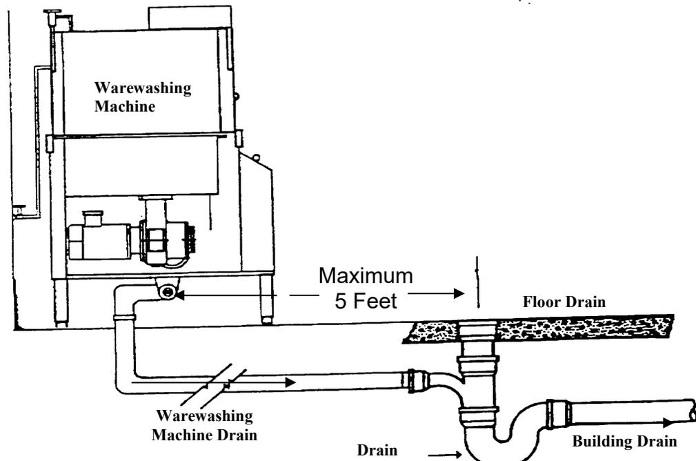
3. Other examples of required indirect drain line connections are:
