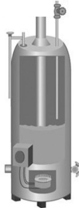
*They slowly heat cold water at the bottom of the tank as stored heated water at the top of the tank is depleted by demand from fixtures and equipment. If sized correctly to all installed fixtures and equipment, it will provide a constant amount of hot water at fixed rate in gallons per hour. They operate by stored water temperature and they burn energy often to maintain a set temperature in the storage tank whether or not hot water is being demanded by fixtures and equipment.*
