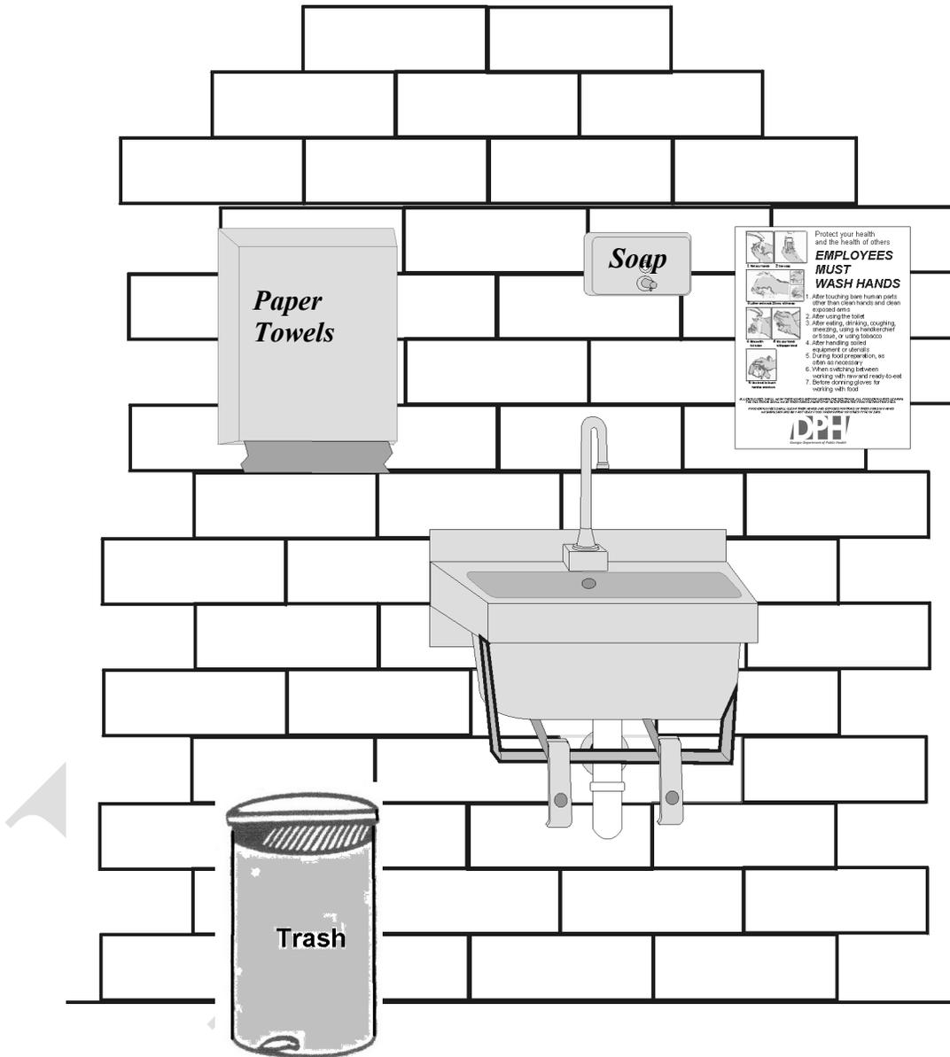
*Handwashing Sink with knee pedestals for water activation*
