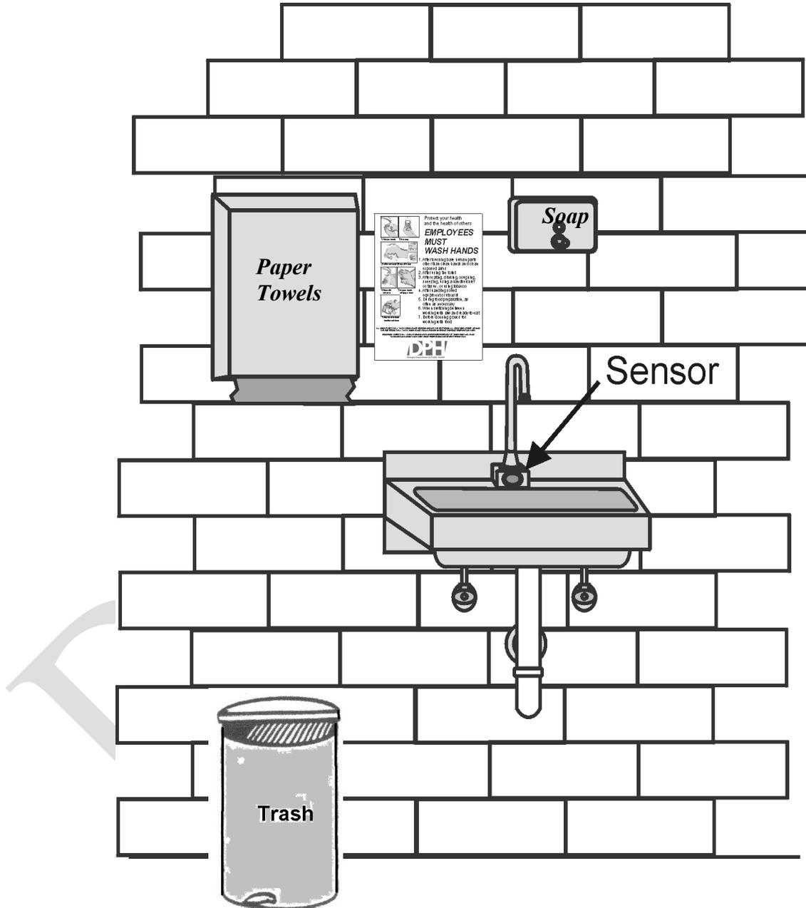
*Handwashing Sink with infrared sensor for water activation.*
