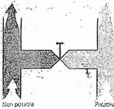
FIGURE 11. Valved connection between potable water and sanitary sewer.
