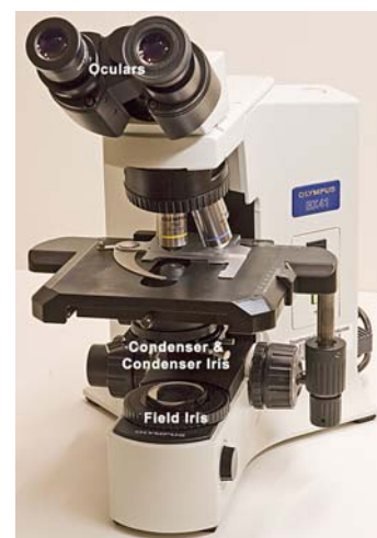
Microscope parts involved in Kohler illumination
