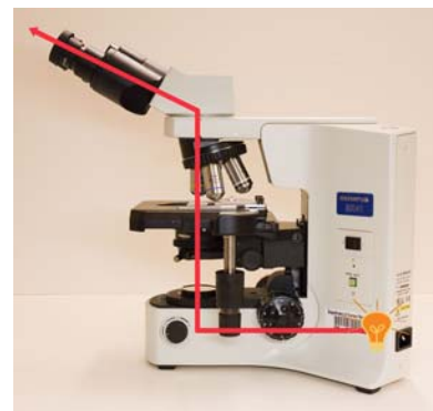
Compound microscope light path
